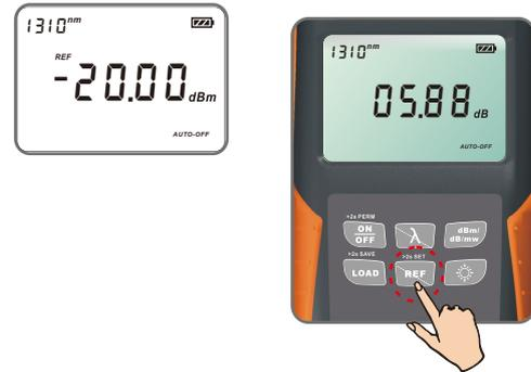
2. Press and hold the “REF” key over 2 seconds to store the presently measured value as the new reference level for the current wavelength. During the process the “REF” sign flashes twice on the screen and buzzer sound is heard. Once the new reference level is set, the FHP2 switches to the dB measurement mode. The displayed value only lasts 1 second.
