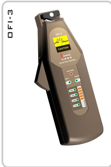
The OFI-3 optical fiber identifier is an inexpensive, portable instrument designed to identify optical test tones and live traffic without disconnecting live system. By simply clamping the OFI-3 onto a fiber, the instrument will indicate if there is a signal, or traffic and show the signal direction. It can detect a variety of optical tones, 270Hz, 1KHz and 2KHz.
