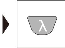
Press the “λ” Key to switch the wavelength between 1310nm and 1550nm(FHS1D02), 850nm and 1300nm(FHS1D03).
