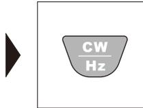
The instrument defaults to CW when it switch on. When it is set to CW, there is no frequency on display. Press the "CW/Hz" Key to select the output among 270Hz, 1kHz and 2kHz.
