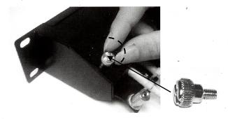
Place the metal cover onto the bottom case and fasten screws.
