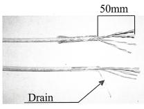
Strip approximately 50mm from the cable jacket, fold back the foil or braid shield, and separate the wire into 4 pair each.
