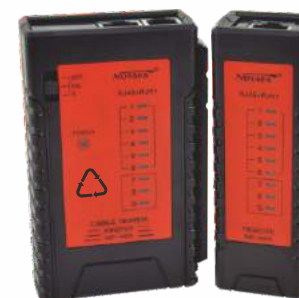
NF-468:verify RJ11/RJ45 Cable
