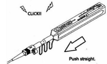
Be careful not to slant the Smart Cleaner SC while inserting into the adaptor.
