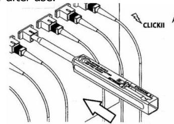
Be careful not to slant the Smart Cleaner SC while inserting into the adaptor.
