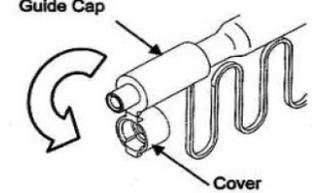
2. Insert SC connector into the Guide Cap.
