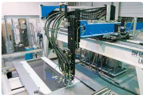
Centre for glass gluing and cabinet door seal applications
