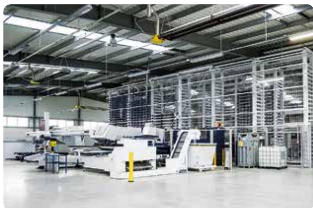
Combined machine - laser and punching
