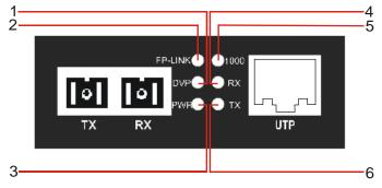
Table 2: Front panel for dual fiber media converter
